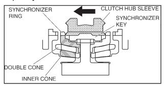
1. When the hub sleeve moves to the left (in the direction of the arrow), the synchronizer key presses against the synchronizer ring.
