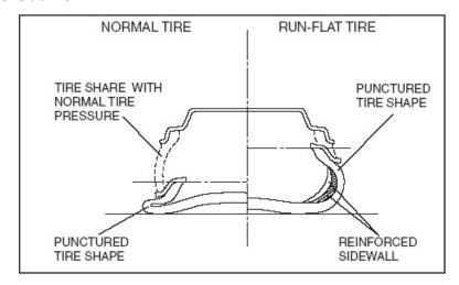
Because the run-flat tire sidewalls have been reinforced, vehicles with run-flat tires can be driven for 80 km (49.6 mile) at 89 km/h (55.2 MPH) even with air leakage caused by tire damage.
