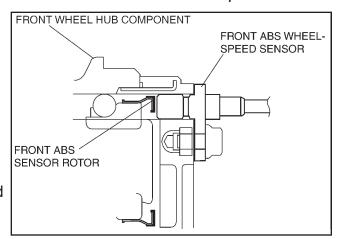
any malfunction of the front ABS sensor rotor, replace the wheel hub component.
