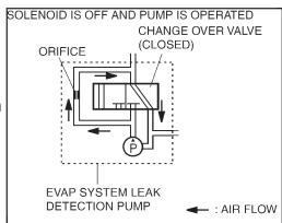
The leak detection pump draws air from the air filter and sends it to the charcoal canister to pressurize the evaporative system.
