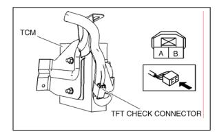
12. Shift from N to D and D to N within 1.5s as illustrated in the diagram. Be sure to end the cycle in the N position and watch the AT warning light in the cluster.
