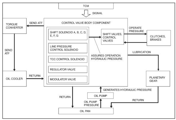
The control valve body supplies oil by switching the oil circuit for the hydraulic pressure generated by the oil pump. Based on the control signal from the TCM, the solenoid valves are activated to control the hydraulic pressure to the clutch and brakes, performing gear shift and TCC. In addition, an appropriate amount of oil is supplied to the torque converter, planetary gears and lubricating parts.
