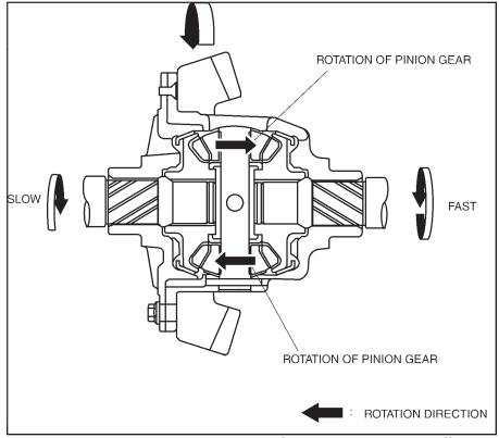
• If the rotation speed between the right and left wheels becomes different (during normal driving), the pinion gears rotate together while revolving around the center axle of the drive shaft, thereby absorbing the difference in rotation speed. This mechanism serves as a differential.
