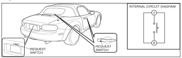
Installed on both doors and trunk lid.
