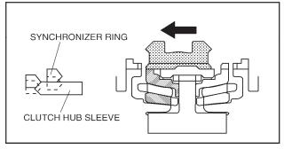
4. The hub sleeve then engages the synchro teeth of the gear to complete shifting.
