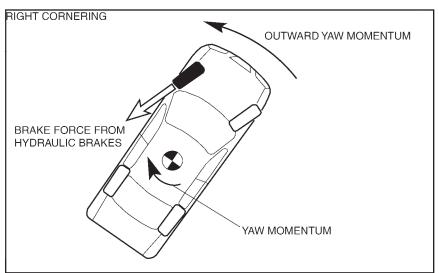
When a large oversteer tendency is determined, braking is applied the outer front wheel according to the degree of the tendency. As a result, a yaw moment is formed towards the outer side of the vehicle and the oversteer tendency is suppressed.
