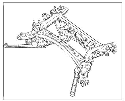
• Adoption of a six-point mounting system rear crossmember ensures link support stiffness and isolates vibration, improving riding comfort and reducing road noise.
