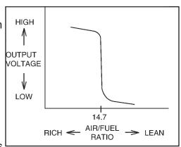
significantly at the boundary of the stoichiometric air/fuel ratio (A/F=14.7). The PCM receives the voltage generated from the HO2S directly, and increases or decreases the fuel injection amount by the fuel injection control so that it is close to the stoichiometric air/fuel ratio.
