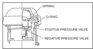
Under normal operation conditions, evaporative gas is vented through the twoway check valve built into the rollover valve. The positive and negative pressure valves in the fuel filler cap have higher opening pressures than the two-way check valve, so they are normally closed. The valves will open if the evaporative pressure inside the tank is too high.
