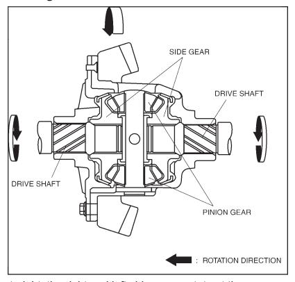
When driving straight, the right and left side gears rotate at the same speed, and the pinion and side gears rotate together with the differential gear case. Input force from the ring gear is transmitted to the pinion gears via the gear case and to the drive shaft via the side gears. Due to this, a speed difference between right and left in the differential does not occur.
