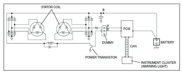
The phase difference in the circuit of the two stator coils causes the electromagnetic pull between the rotor and the stator to be eliminated logically. Due to this, electromagnetic vibration and generator operation noise (electromagnetic noise) have been reduced.
