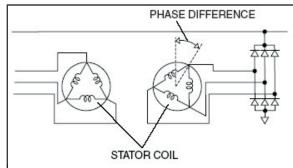
• The pulsation occurring through voltage rectifying is minimized, as a result, stable voltage output is supplied due to the adoption of two stator coils with the phase
