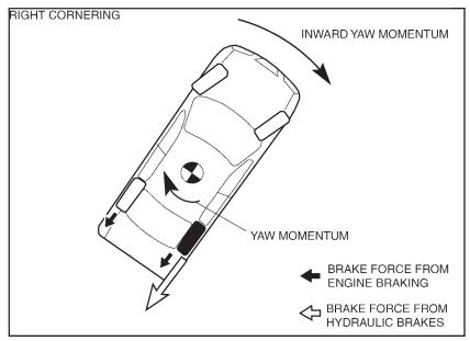
When a large understeer tendency is determined, engine output is controlled and braking is applied to the inner front wheel according to the degree of the tendency. As a result, a yaw moment is formed towards the inner side of the vehicle and the understeer tendency is suppressed.
