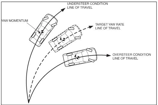
The vehicle speed, steering angle, lateral-G and yaw rate are detected by the sensors and used in calculations by the DSC HU/CM to determine the vehicle condition. Then, depending on the difference between the target yaw rate, calculated with the values input from each sensor, and the value detected by the yaw rate sensor, an oversteer or understeer tendency can be determined.
