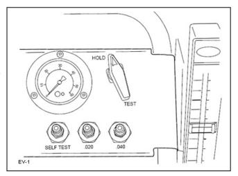
6. Verify the gauge holds pressure and that the flow meter reads "no flow". No flow indicates the tester passed self-test. If the tester didn't pass, contact the instructor.
