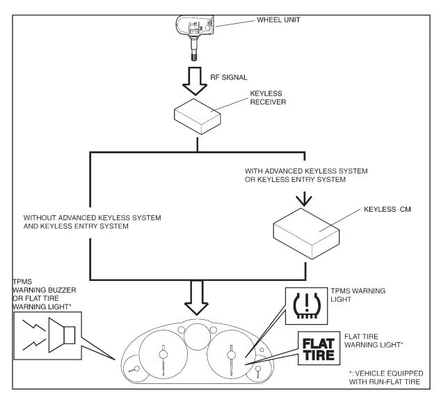
The TPMS consists of wheel units that detect air pressure, temperature and acceleration of each tire, and a TPMS control module that receives data (RF signals) sent from the wheel units to monitor the air pressure of each tire.
